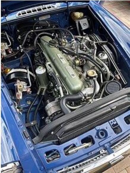
Most MGCs came to North America with this configuration – emission control, dual brake circuits etc.
