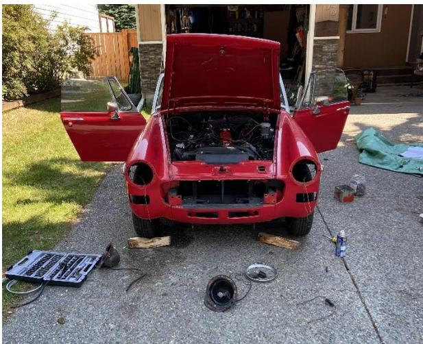
cylinder pumped fluid everywhere but to the clutch. Moss Motors to the rescue – Connor ordered new lines and hoses – Moss got the parts right on the second try. The next step was to bleed the circuit, but this also included bleeding and renewing the brake hydraulics as well. Enlisting some assistance from friends, and an older neighbor who it turned out had considerable mechanical experience with British cars, Conner
