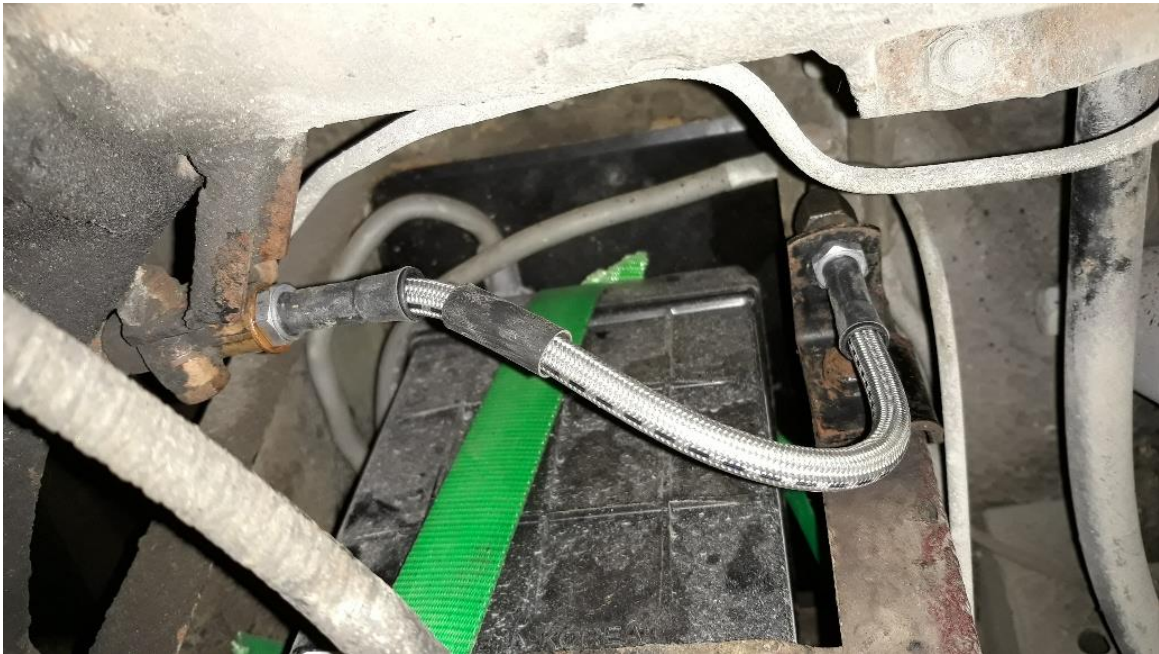
View of the new stainless braided hose after installation. It is located in the tight space between the battery and rear axle.
