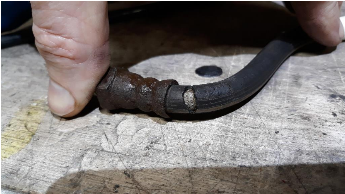
Original rear rubber hose showing the perished and cracked casing
