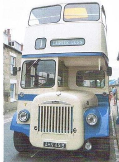
*Mid '50s Daimler CCG5 bus. It had a 5 cylinder Gardner diesel engine and 4 speed Guy crash gearbox*
