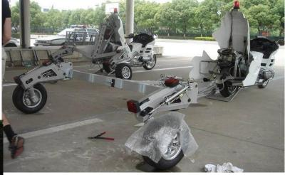
The trailer has a 3 wheel design that isolates the bike from the weight of the car and allows the bike to corner naturally. The trailer is also fitted with its own brakes to assist with safe transport of the car and rider. The trailer is hydraulic powered and just needs to be fitted around the car and then raised before it is secured.
