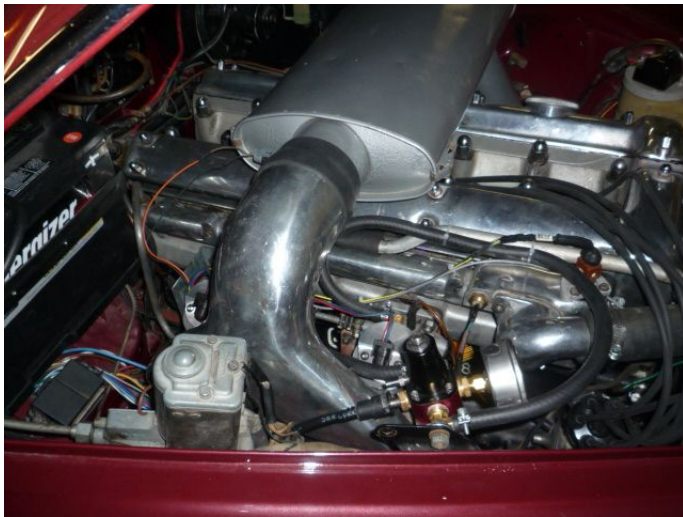
Figure 3: The completed underhood installation of all sensors and fuel components.
