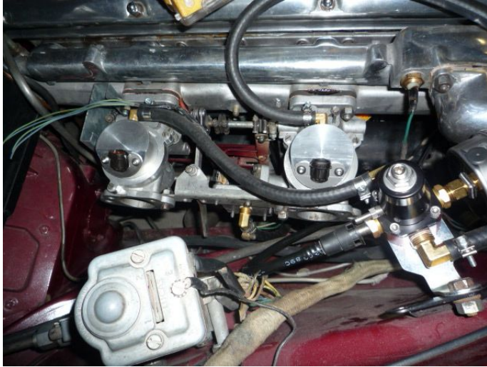
Figure 2: The carb adapters in place with injectors installed. The adjustable fuel pressure regulator is on the original fuel filter bracket.
