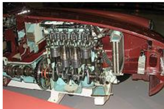
A sectioned MGB showing engine and gearbox configuration
