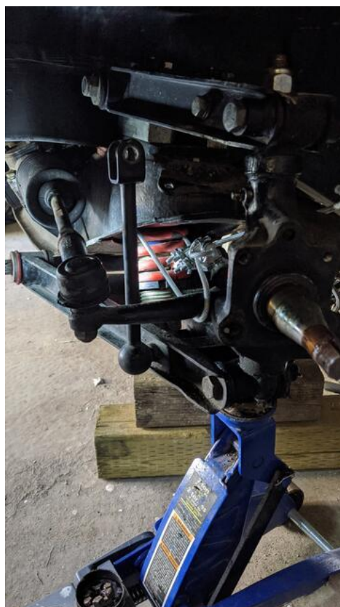
Aircraft Cable in place to prevent explosive disassembly of the suspension and allow removal of the broken shock
