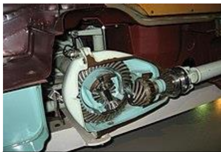
A sectioned MGB showing the rear axle and differential
