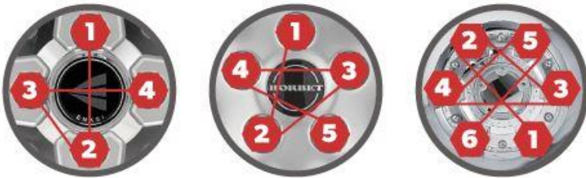
Tightening and Loosening Patterns
