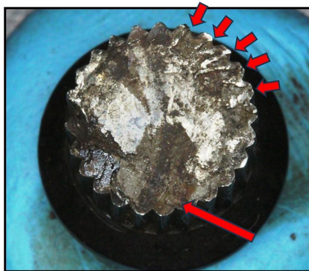
Stud head fracture surface
