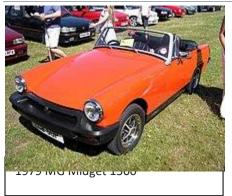
To meet US federal regulations, large black plastic-covered bumpers were added to the front and rear and the ride heights were increased. The increased ride height affected handling and anti-roll bars were added to help with the higher centre of gravity.
