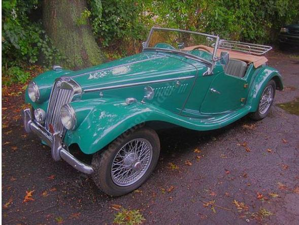
The TF Midget, launched on 15 October 1953, was a facelifted TD, fitted with the TD Mark II engine, headlights faired into the wings, a sloping radiator grille concealing a separate radiator, and a new pressurized cooling system. The styling changes were to make the car look more modern.
