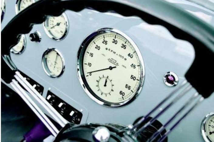
The instrument panel itself was re-created out of a single sheet of aluminum, to match the rest of the car's stunningly seductive skin. The design and layout of the dashboard came courtesy of a period photograph of the car's interior, which showed the proper location of all the gauges.
